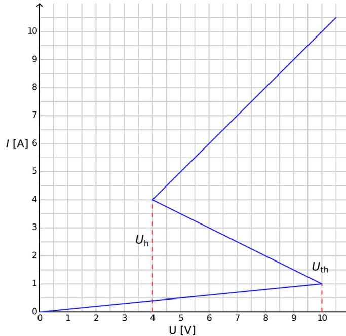
Figure 1 (圖 1) :  $I - V$  characteristics of the non-linear element  $X$ .
