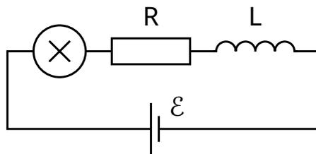
Figure 2 (圖 2) : Circuit with element  $X$ , resistor  $R$ , inductor  $L$  and voltage source  $\mathcal{E}$ .
