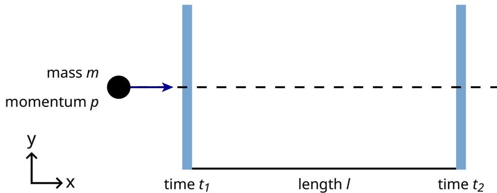
Figure 2 (圖二) : Schematic view of a time-of-flight detector.
