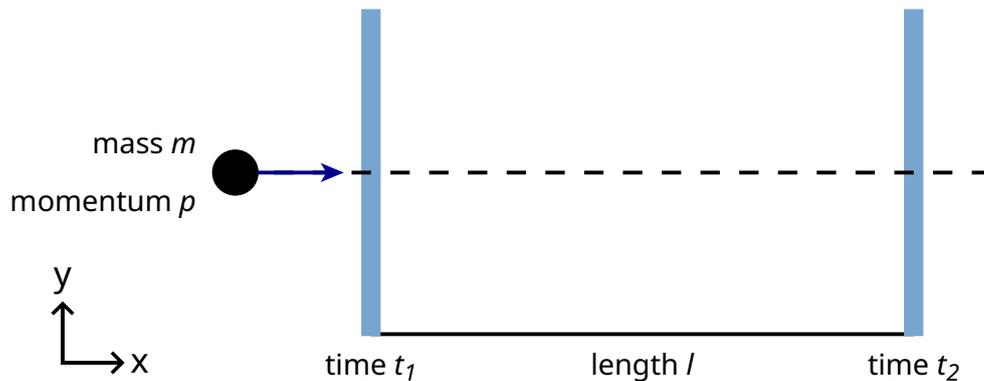
Figure 2: Schematic view of a time-of-flight detector.
